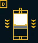
The system pressure falls and pressurized gas in the accumulator forces the fluid from the accumulator back into the system.
