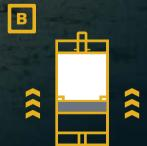
The hydraulic system is pressurized. The system pressure exceeds precharge pressure, and the fluid flows into the accumulator.
